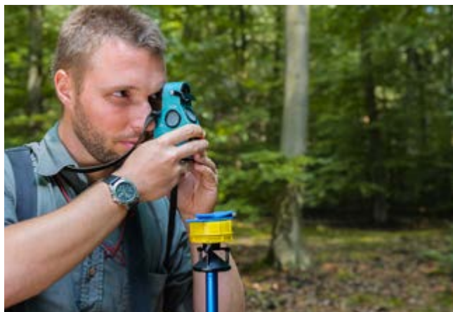
The sample trees for angle-count sampling are determined using a Bitterlich relascope and ultrasonic distance-measuring device.
