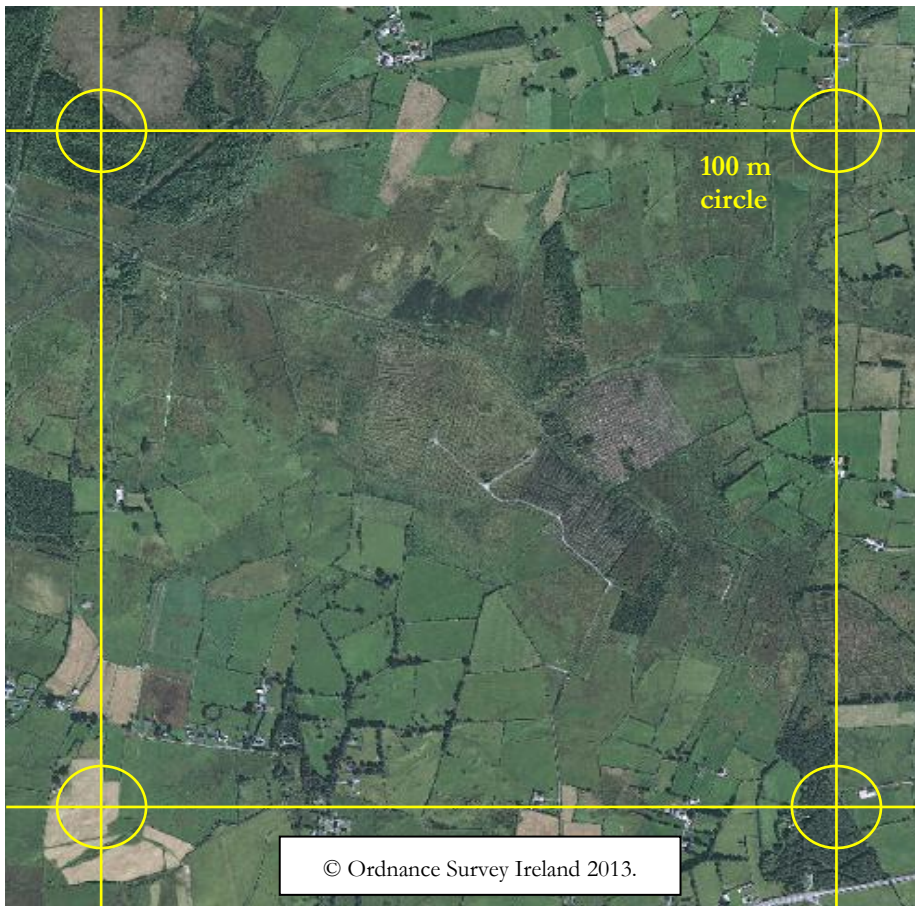
Figure 3. Location of sample plots is randomised within 100m of 2km systematic grid.
