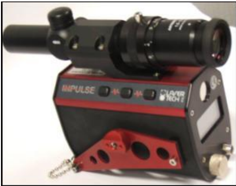
Figure 93. Impulse™ laser range finder and remote diameter scope.
