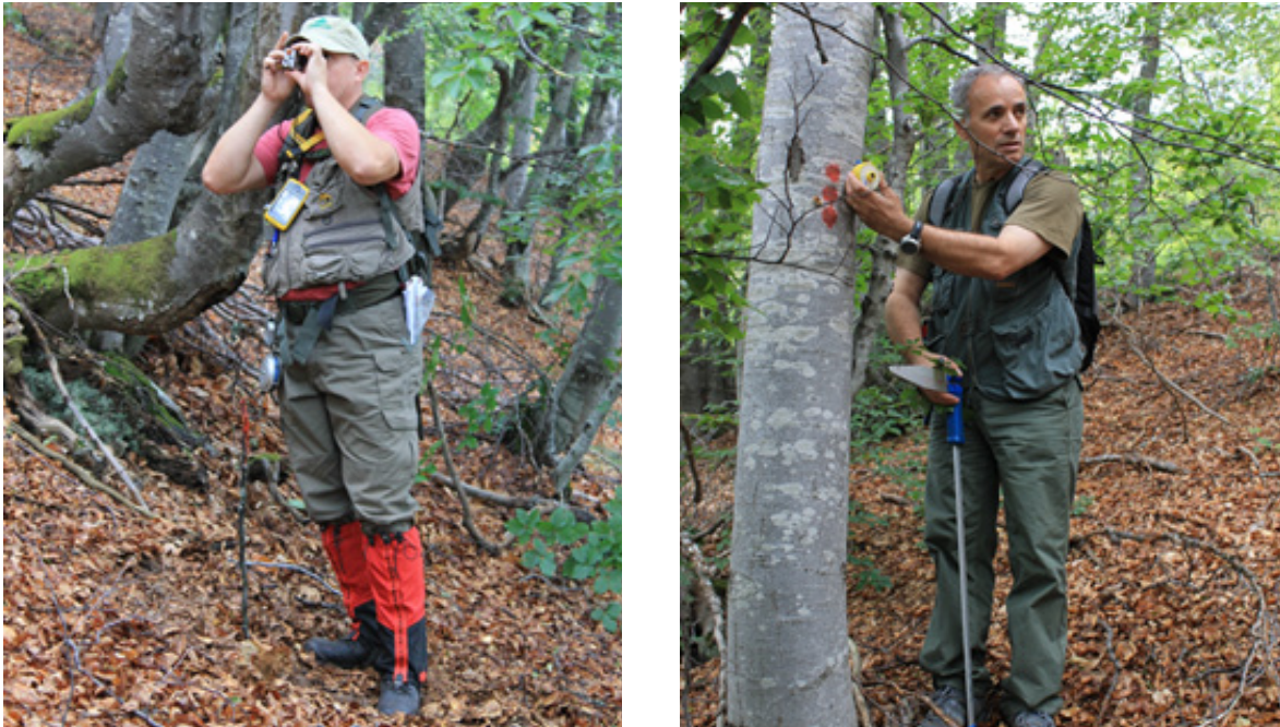
Figure 8: Fieldworkers measuring height of sample trees using Vertex hypsometer (left) with transponder (right)
