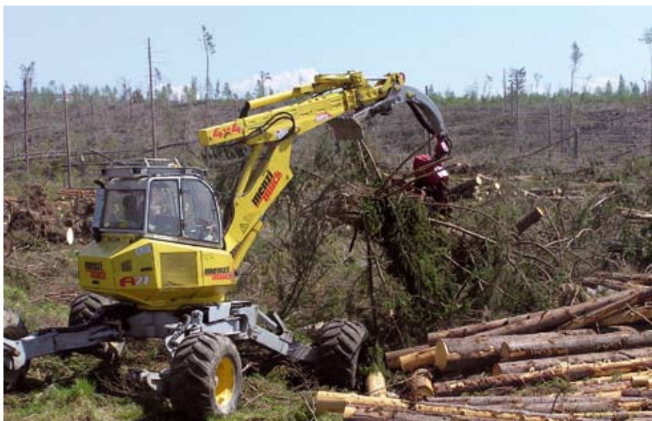
Figure 30 Harvester Menzi Muck A71 in a windthrow affected area
